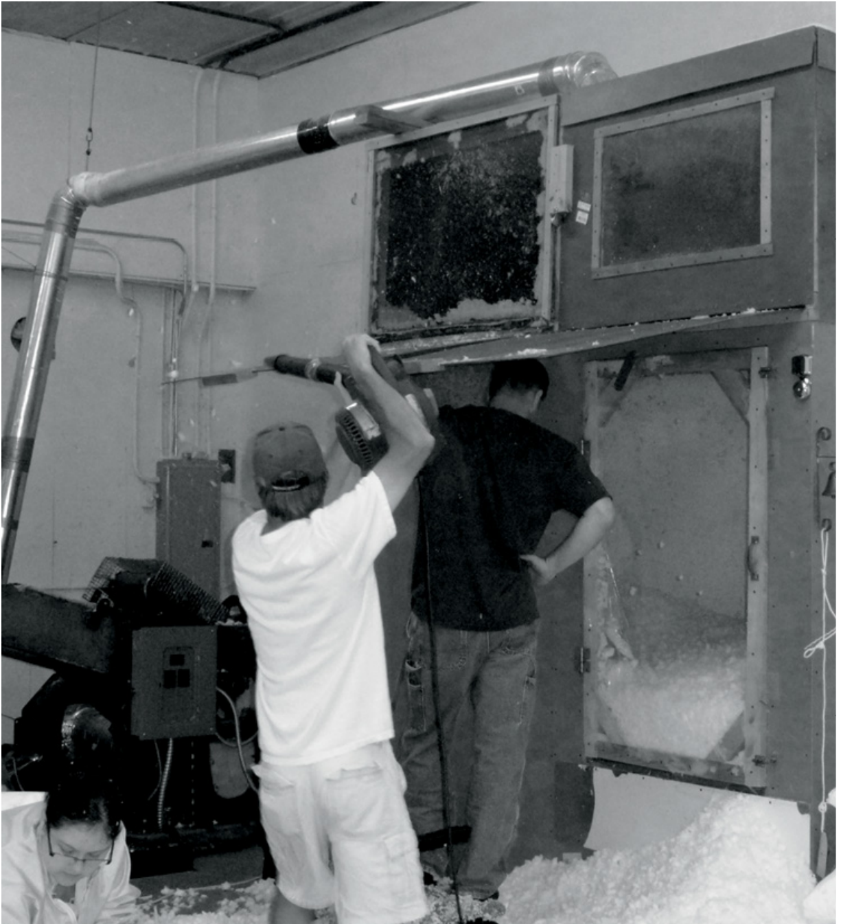
2005 I built this bin and added it to the foam grinder to capture the shredded foam.
